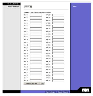
Figure 6-11: Wireless - Wireless MAC Filter Screen
